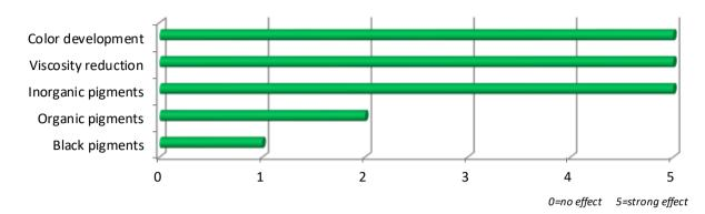
UNIQ®SPERSE P-190 is a wetting and dispersing additive for filled unsaturated polyester. The dispersant is especially suitable for inorganic pigments and filler pigments. Strong viscosities reduction so higher pigment and filler loading in the grinding process can be achieved.
